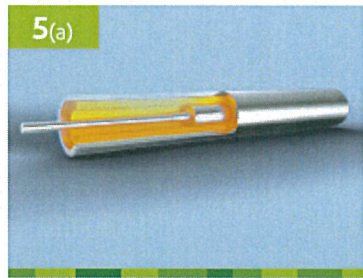
5(a) Piercing of billet at piercing press
