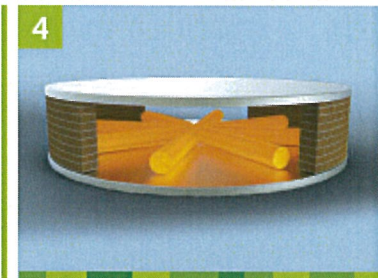
4 Heating of billet in rotary furnace
