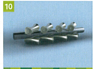
Straightening of pipes
