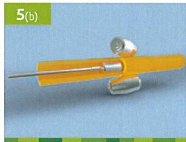
5(b) Piercing of billet at cross-roll piercer
