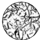
Gray Iron Excellent castability but 'brittle' – less strength
